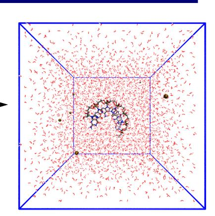
MD simulation Water: TIP3P, RNA: Amber14Sb Simulation time: 100 ps
